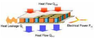
Pictures: Design/Function Thermoelectric generator, Jihui Yang GM DEER 2006
