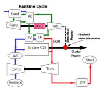
Picture: Caterpillar layout for HECC HPL EGR waste heat recovery system – Rankine
