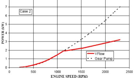
Power consumption standard gear pump and variable flow pump Source: www.concentric-pump.co.uk
