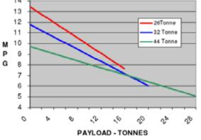
Figure: Effect on Payload on Fuel Consumption Based on 3 Different Trucks Reproduced from [1]
