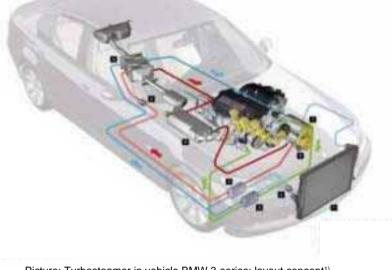
Picture: Turbosteamer in vehicle BMW 3-series; layout concept<sup>1)</sup>
