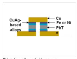
Picture: Layout thermoelectric generator, Ed Gundlach GM DEER 2008
