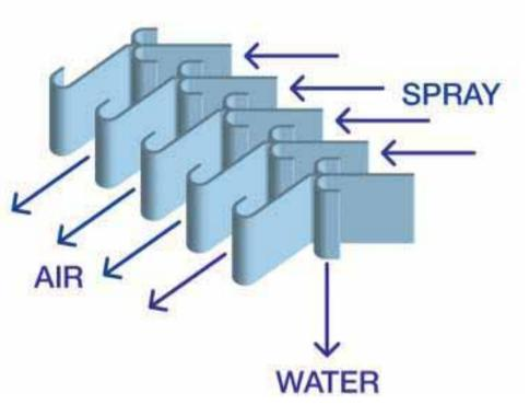
Operation principle of Spraydown technology
