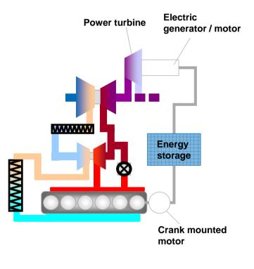
Picture: Turbogenerator – system layout
