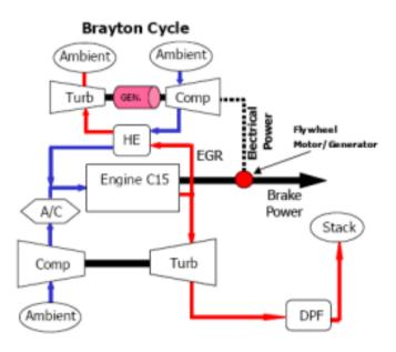
Picture: Caterpillar layout for HECC HPL EGR waste heat recovery system – Brayton  $^{1)} \$
