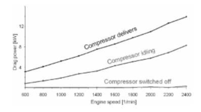
Drag Power Compressor with Shut-off Clutch Picture: Schaller K V, MAN, Aachen 16 Kolloquium, 2007
