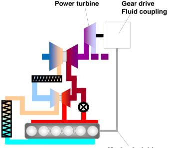
Mechanical drive to crankshaft
