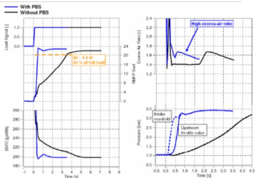
Picture: Tested PBS system at 1000rpm load response (blue PBS ON - black PBS OFF) Knorr-Bremse; 29th IWM, 2008 30)
